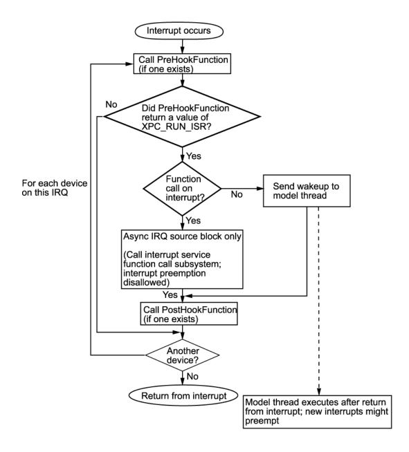
When a device interrupt occurs, the generated code uses the following steps for each device on this IRQ to determine which device generated the interrupt:
